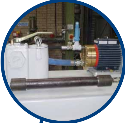
Dust Suppression Pumping water or latex emulsions for airless spray
