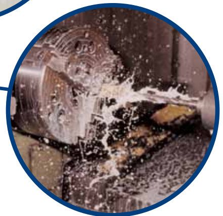
Deep hole drilling
