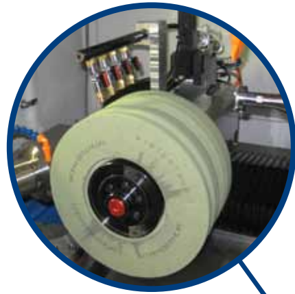
Grinding Wheel cleaning/dressing
